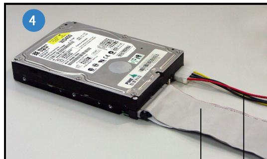
IDE ribbon cable Power cable
